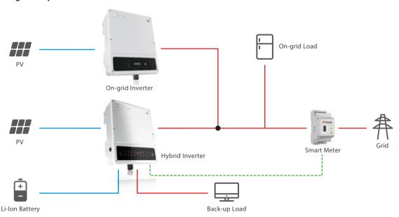
This solution integrates both hybrid and retrofit functions into a single system. In both on-grid systems as well as hybrids, the solar energy is used to supply electricity to both back-up loads and to charge the battery before the power is injected into the grid. By adopting such a solution, the system provides a more reliable source of supply for the loads, while ensuring a sufficient supply of green energy to charge the battery.
