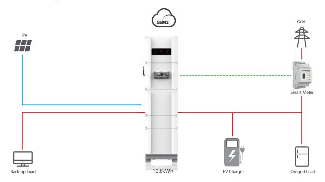
GoodWe is pleased to introduce the ESA Series, an "All-in-One" hybrid system that is designed to simplify the installation process to the maximum. It consists of the following elements: a hybrid inverter, a battery bank and a pre-wired system located inside a modern cabinet; it also includes connection devices and a preset cable slot. It is estimated that this system reduces the installation cost by as much as 60%!
